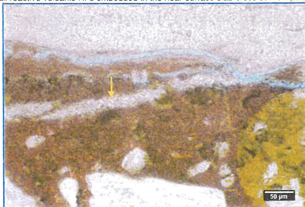
2D. Detail of the crack-filling amorphous metasilicate gel (yellow <).
