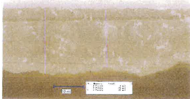
Figure 14. Microscope image at 200X magnification showing SignaFlor core #3 in cross-section with moisture mitigation membrane intact (bottom layer). The membrane had debonded from the concrete and the intact core was easily removed. The uneven surface is the epoxy/concrete interface showing adhesive failure.
