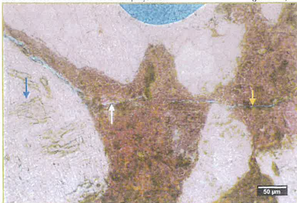
3D. Detailed view of the highlighted area from 3C. The fractures and cracks are locally filled with metasilicate gel (white <) and have weakened the cohesive integrity of the substrate surface.
