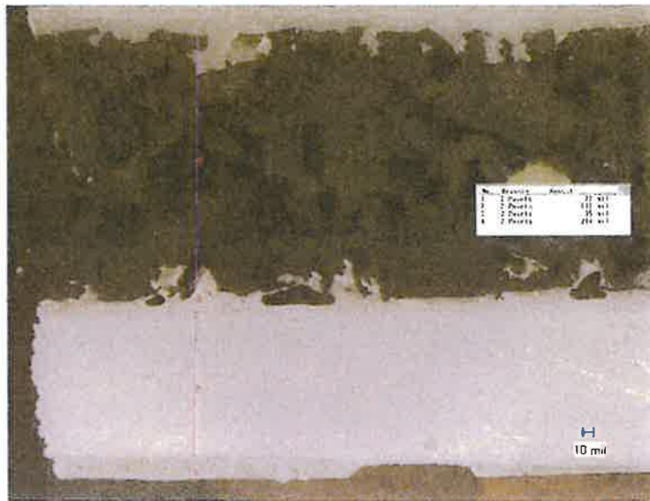
Figure 11. Microscope image at 20X magnification showing a cross-section of the lower portion of SignaFlor core #1. The black layer is the rubber base mat. The moisture mitigation membrane was strongly adherent to the concrete slab. The smooth surface (bottom) is where the SignaFlor system split during forceful removal of the SignaFlor core sample.
